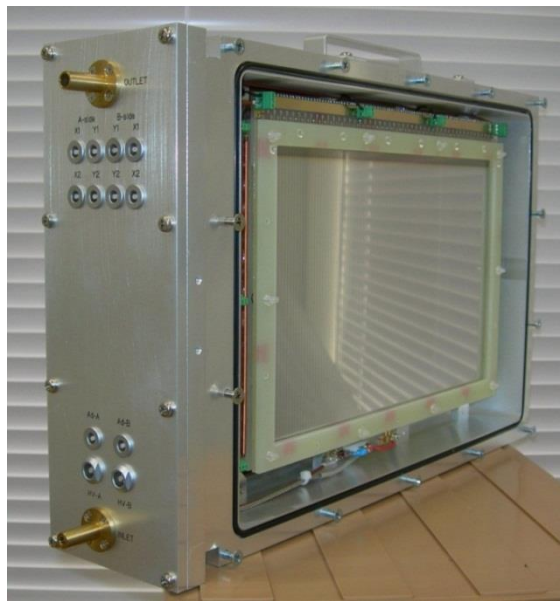
Fig. 7. Photograph of the 240 mm (X) \times 150 mm (Y) double PPAC detector.
